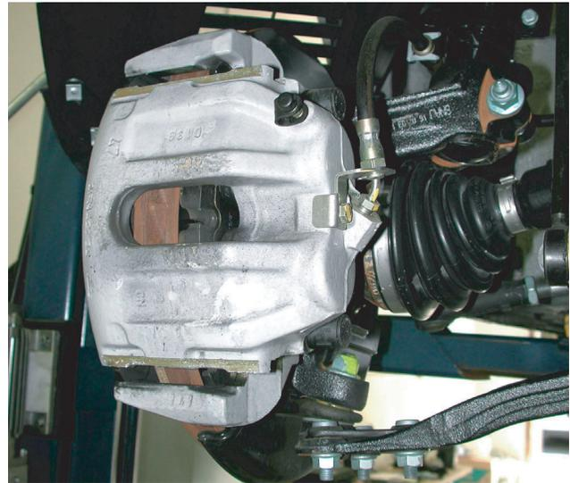
Front Wheel 2FN Dual-Piston Floating Frame Calipers
