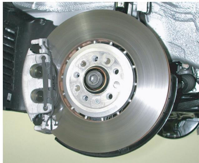
Front Wheel Two-Piece Ventilated Directional Rotors
